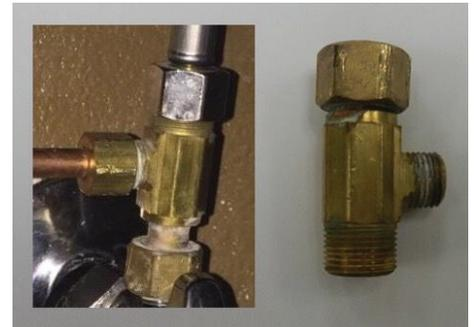
This small brass tee under a kitchen sink was all it took to raise lead leaching to an extremely high level. Once replaced, the water was re-tested, and shown to be well below the EPA cutoff of 15 ppb.
